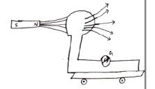
slow, the deflection in galvanometer is small. Hence greater is the rate of change of magnetic flux linked with the coil greater is the induced current set up in the coil.
