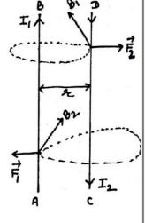
Again according to Fleming's left hand rule, this force acts at right angle to AB, toward CD in the plane of the paper. Thus when the current in the two wires are in same direction, the force is attractive & when current are in opposite direction, force is repulsive.
