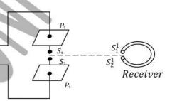
When input is supplied then spark produces between metallic plates which produce electromagnetic waves of frequency  $v=\frac{1}{2\pi\sqrt{LC}}$
