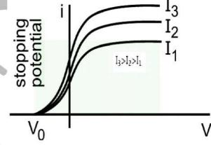
If anode is connected to -ve terminal of the battery then current decreases and at a certain -ve potential of plate A, the current becomes zero.
