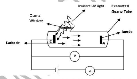
The experimental setup used to study the photoelectric effect is consisting of a vacuum tube having two metallic electrodes A and C.
